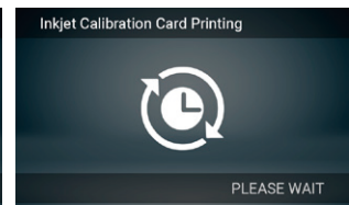
4. The printer will print the calibration card automatically. This takes approximately 15 minutes. (Make sure you have loaded the filament.)
