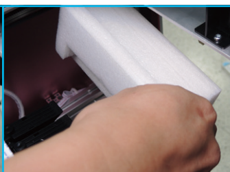
9 Remove the cable tie and foam in front and back of the front door.
