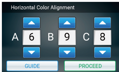
6. For horizontal alignment, enter each color's corresponding number. After entering the number, tap PROCEED.
