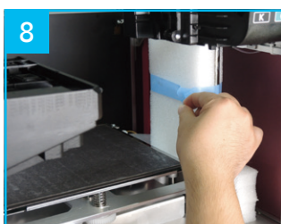
8 Remove the foam next to the guide screws on both sides, and then remove the foam under the print bed.
