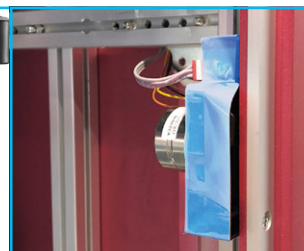
5 Open front door, remove the tape at mark printer door post.
