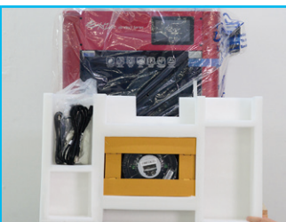
3 Remove the packaging materials, top cover box, accessory box and plastic cover.
