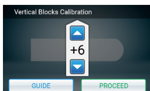
7. Vertical direction: Enter the number of the box you think the filament and ink align the most, and then tap PROCEED.
